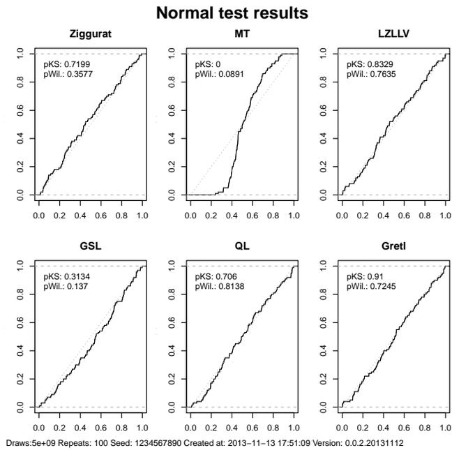
Figure 5: Standard Test applied to Ziggurat generators
